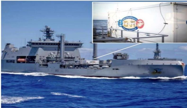
A server rack containing three independent optical clocks, a 1-U power supply, a control laptop for each clock, an uninterruptible power supply, and a measurement system were loaded in a total rack volume of 23 U. The cargo container housing the rack was craned onto the deck of the HMN25 Aotearoa, where it remained for a three-week naval exercise. NATURE 628, PAGES 736-749 (2024)
