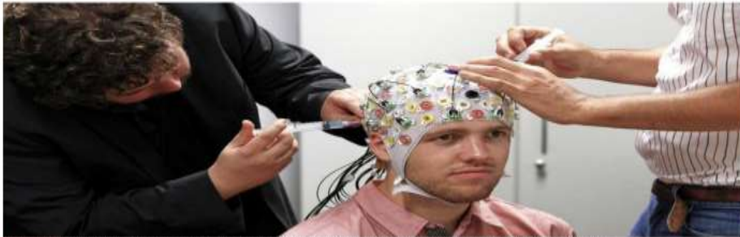
Inside the brain: Researchers inject gel under the electroencephalography (EEG) cap at the Technische Universität München (TUM) in Garching near Munich in 2014. REUTERS
