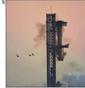
As the booster descends close to the launch tower, the arms (‘chopsticks’) close gently around the booster, catching it before it hit the ground
