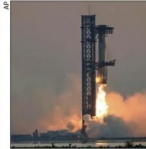
As the booster descends close to the launch tower, the arms (‘chopsticks’) close gently around the booster, catching it before it hit the ground
