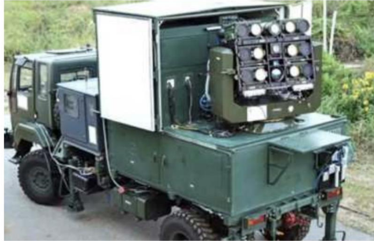
A view of the Laser-Directed Energy Weapon system developed by the DRDO to shoot down aerial targets in Kurnool. ANI X
