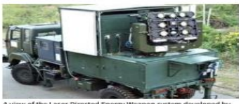
A view of the Laser-Directed Energy Weapon system developed by the DRDO to shoot down aerial targets in Kurnool. ANI X
