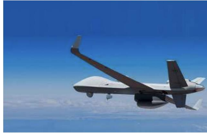
High flyer: The MQ-9B Sea Guardian has a maximum flying altitude of 40,000 feet. SPECIAL ARRANGEMENT
