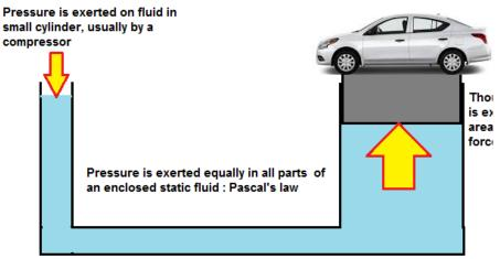
The force in the small cylinder must be exerted over a much larger distance. A small force exerted over a large distance is traded for a large force over a small distance
